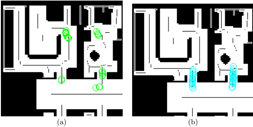
Fig. 5.7. Subfigure (a) visualizes the LOW-T-VEL subtraces of the behavior trace depicted in figure 5.6 and subfigure (b) the subtraces that correspond to the traversal of narrow passages
