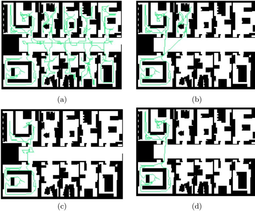
Fig. 6.13. Problem-specific search plans generated by the resource-adaptive, informed search strategy. Subfigure (a) shows an uninformed search plan that searches the region systematically. Subfigure (b) depicts a search path where the robot is told the the target is in one of the three rooms. A search plan that has maximum probability of finding the target within 15 minutes is shown in subfigure (c). Finally, a search path that only searches in three rooms and for 15 minutes is shown in subfigure (d)
