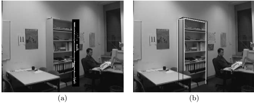
Fig. 6.11. Recognizing the shelf using runtime configured image processing plans. The robot uses context information including its estimated pose, the accuracy of the pose estimation, and the shelf position, to predict where the long vertical lines of the shelf should appear in the image. It generates regions of interest to focus the image processing routines
